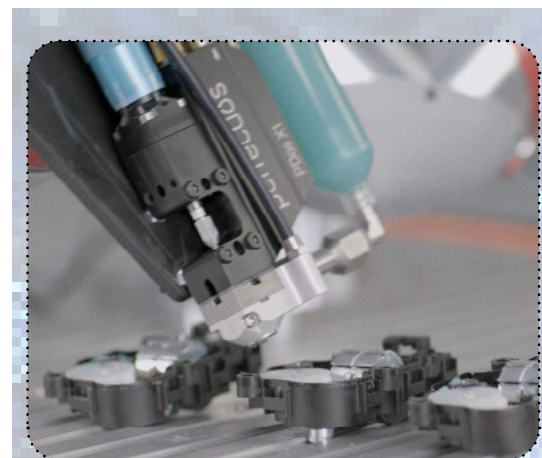
Image 2: With 300 Hz cycle frequency, a high dispensing frequency is achieved at a distance of 50 mm for horizontal and overhead shots (Image: perfectdos GmbH).
